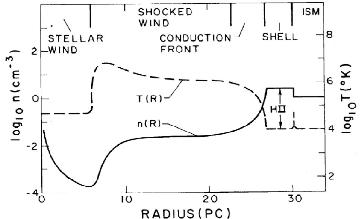
FIG. 3.—The large-scale features of the temperature and density structure of an interstellar bubble for which  $L_w = 1.27 \times 10^{36} \text{ ergs s}^{-1}$ ,  $n_0 = 1 \text{ cm}^{-3}$ , and  $t = 10^6 \text{ yr}$ . ISM means ambient interstellar medium. For a typical O7 I star, the H II region would extend to  $\sim 3 R_2$ .
