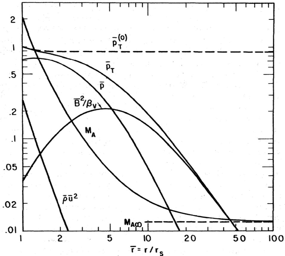
**Figure 8** Solution of equations (34)-(37) with initial conditions determined by equations (30)-(33) and with  $\beta_v = 500$ . Note that the presence of the magnetic field has caused the total pressure  $\bar{p}_T$  to decrease to zero as  $\bar{r} \rightarrow \infty$ , rather than remaining constant ( $\bar{p}_T^{(o)}$ ) as it does in the field-free case [from Cranfill, 1971].
